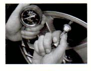
6. Remove the unit by turning the valve stem adaptor in an anti-clockwise direction. Ensure a valve cap is placed on the valve stem to prevent ingress of debris.
